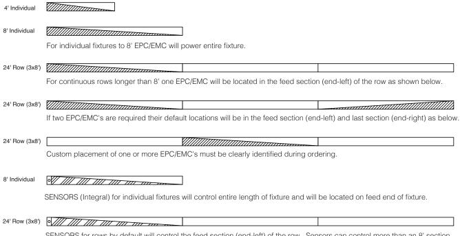
SENSORS for rows by default will control the feed section (end-left) of the row. Sensors can control more than an 8' section within a row. Consult factory for sensor/section options, or for multiple sensors in a continuous row.
