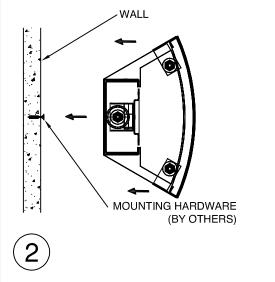
1. INSTALL FIXTURE TO WALL USING APPROPRIATE HARDWARE (BY OTHERS). REFER TO JOB DRAWINGS FOR MOUNTING LOCATIONS.
