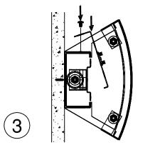
1. FEED SUPPLY WIRES THROUGH HOLE IN FIXTURE. USE APPROPRIATE STRAIN RELIEF TO SECURE FEED WIRES IN FIXTURE AS REQUIRED BY LOCAL ELECTRICAL CODES. STANDARD WIRING DIAGRAM SHOWN, REFER TO JOB DRAWINGS FOR JOB SPECIFIC WIRING
